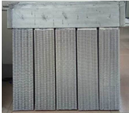
Figure 4 A new type of non-contact high efficient micro heat pipe array
